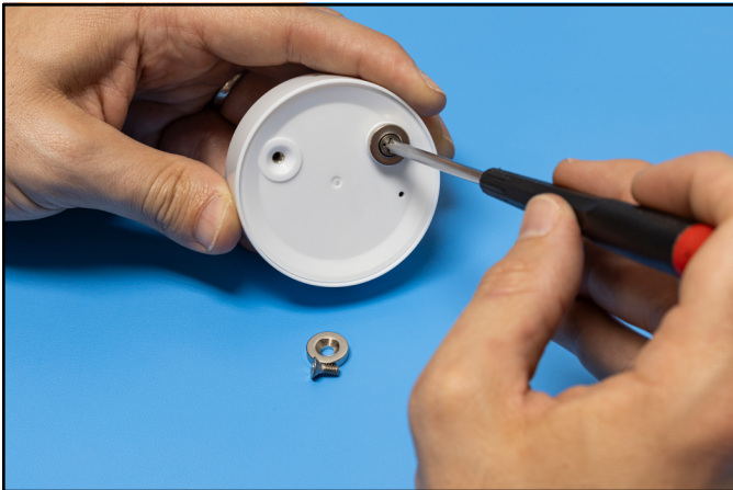
Figure 7. Installing the Desco 19344 Ring Magnets
